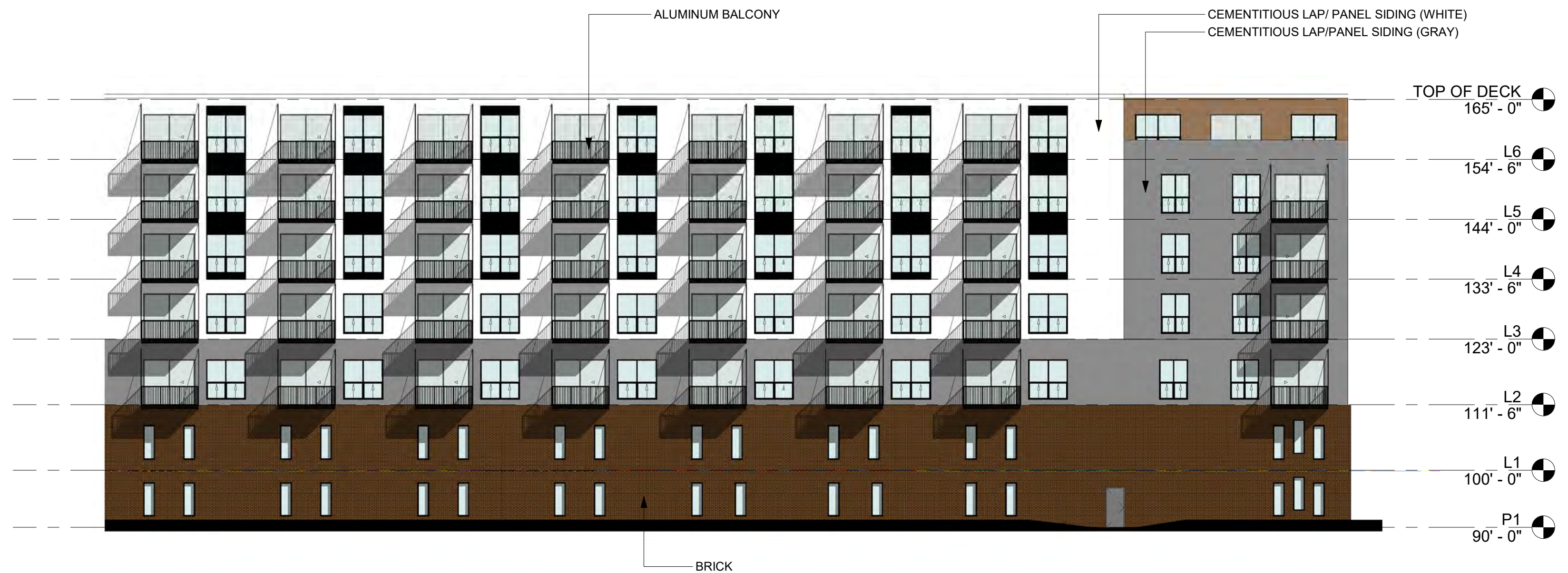
① NORTH ELEVATION - ANGLED 1/16" = 1'-0"
