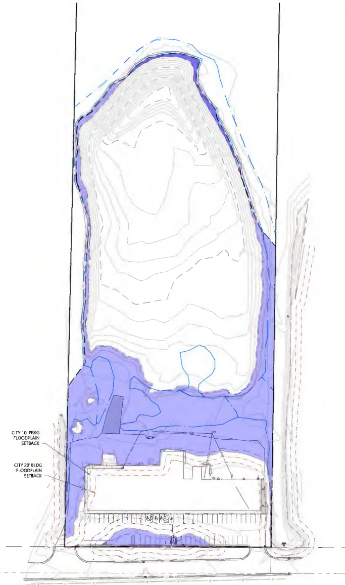
EXISTING FLOOD STORAGE
