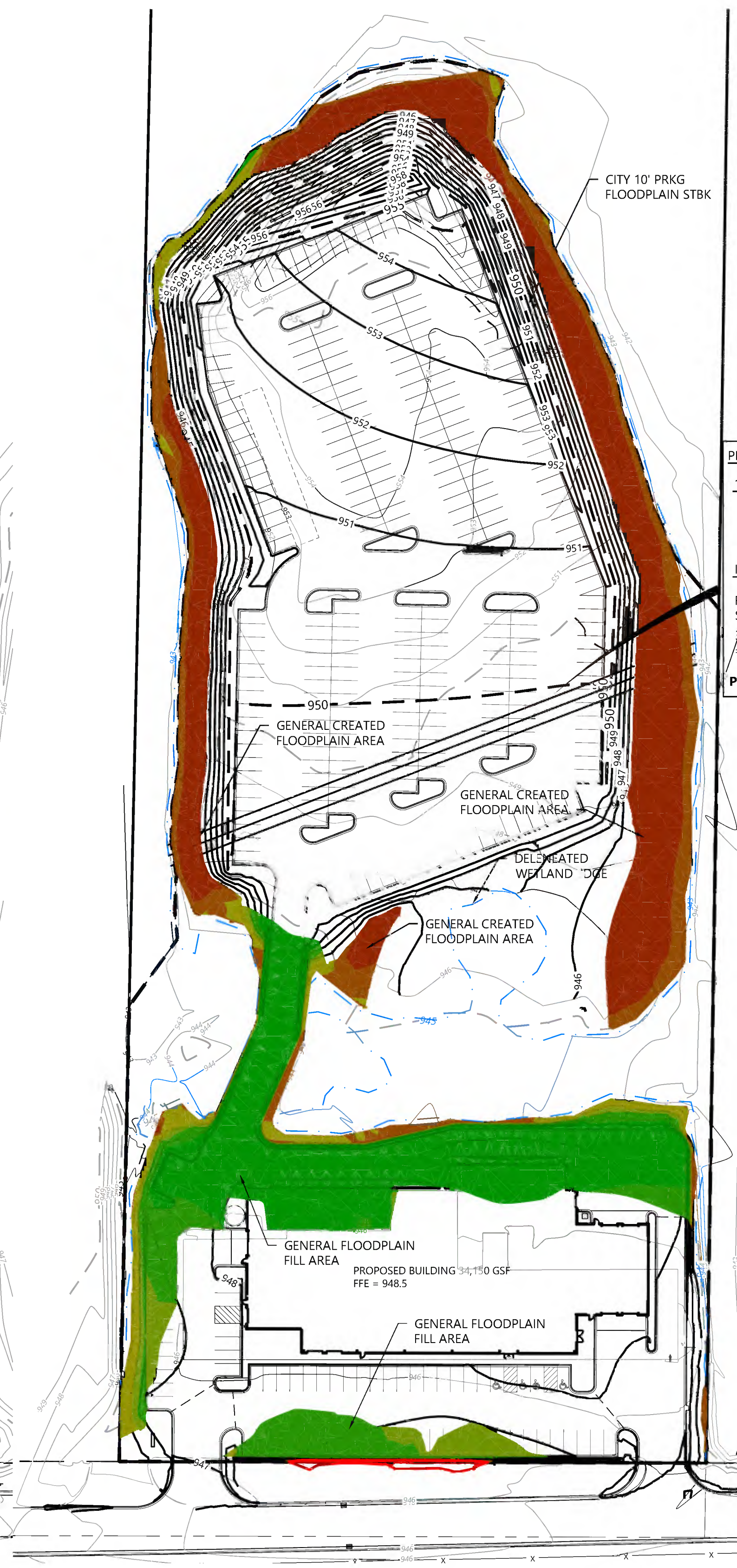
PROPOSED CUT/FILL WITHIN FLOODPLAIN AREAS
