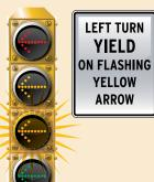
Flashing yellow arrows have proven to minimize delays and enhance safety by reducing driver errors, according to MnDOT.
