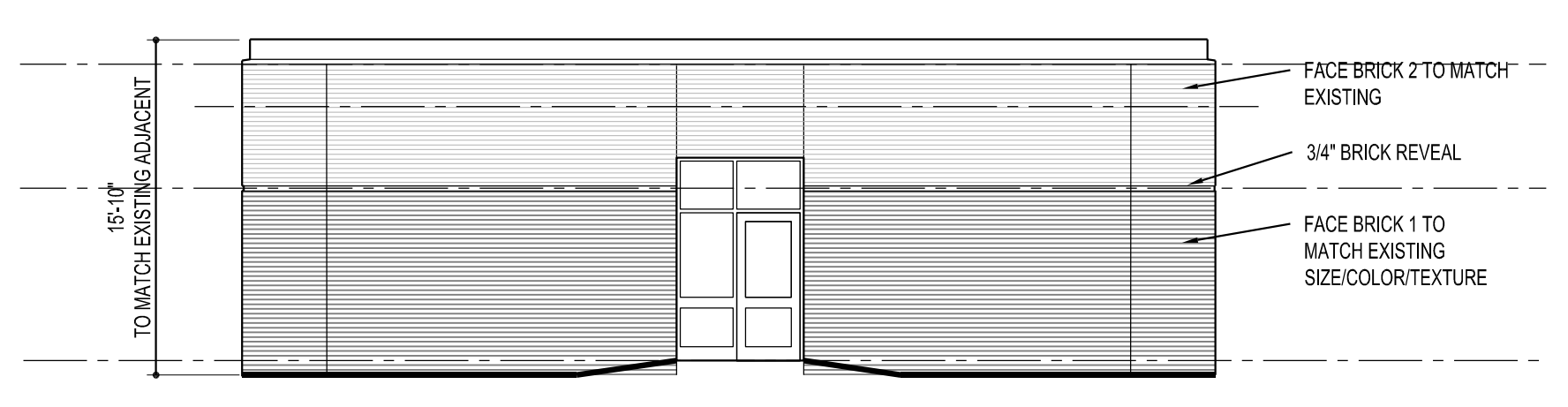
3 EAST ELEVATION UNIT B (ALTERNATE) A1.1 1/8" = 1'-0"
