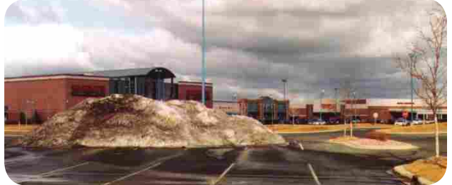
Fig. 70: Snow plowed and piled in parking lot. Consideration should be given to locating these “snow dumps”, since they will contribute a significant amount of stormwater runoff.
