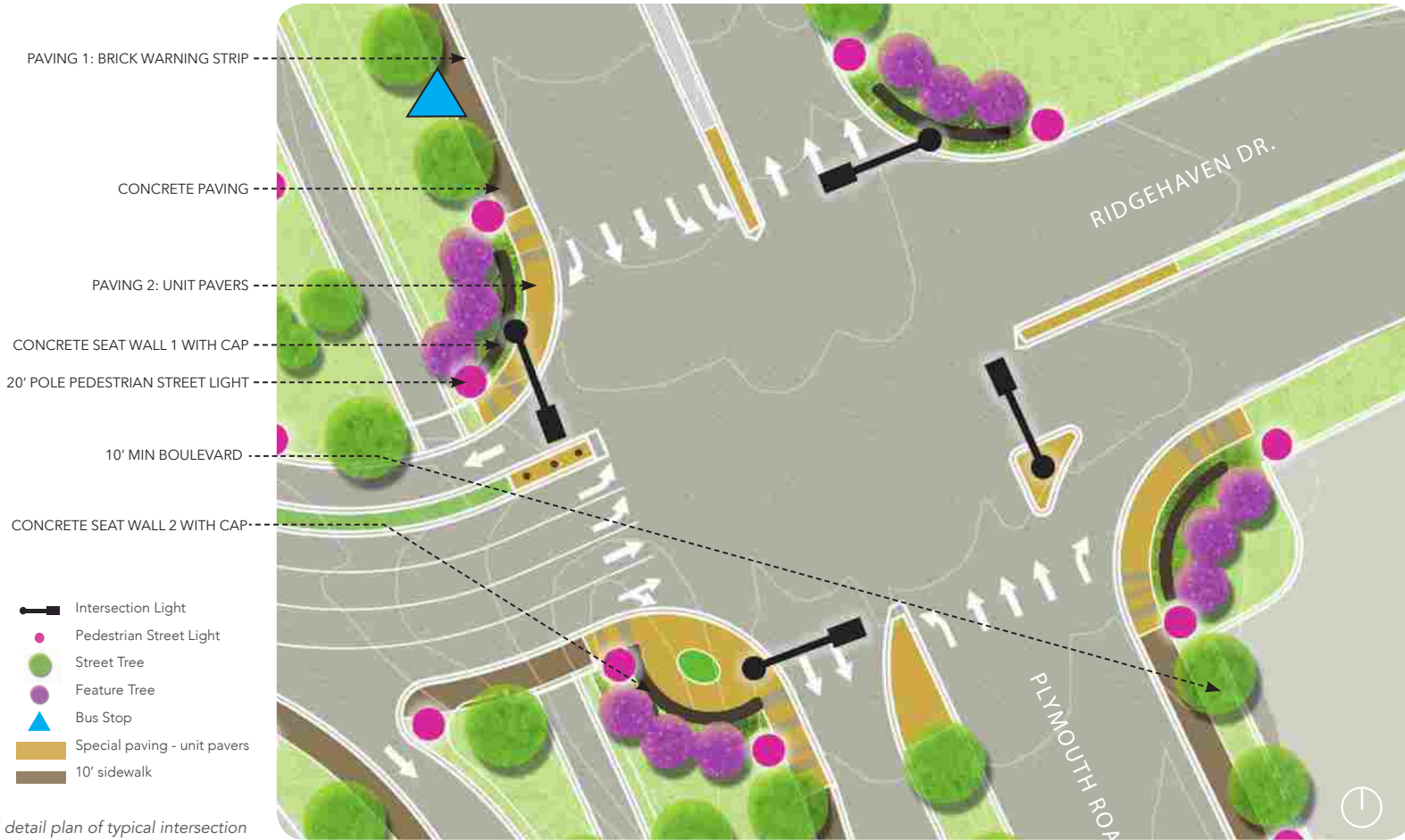
Fig. 37: Proposed detail plan of typical intersection
