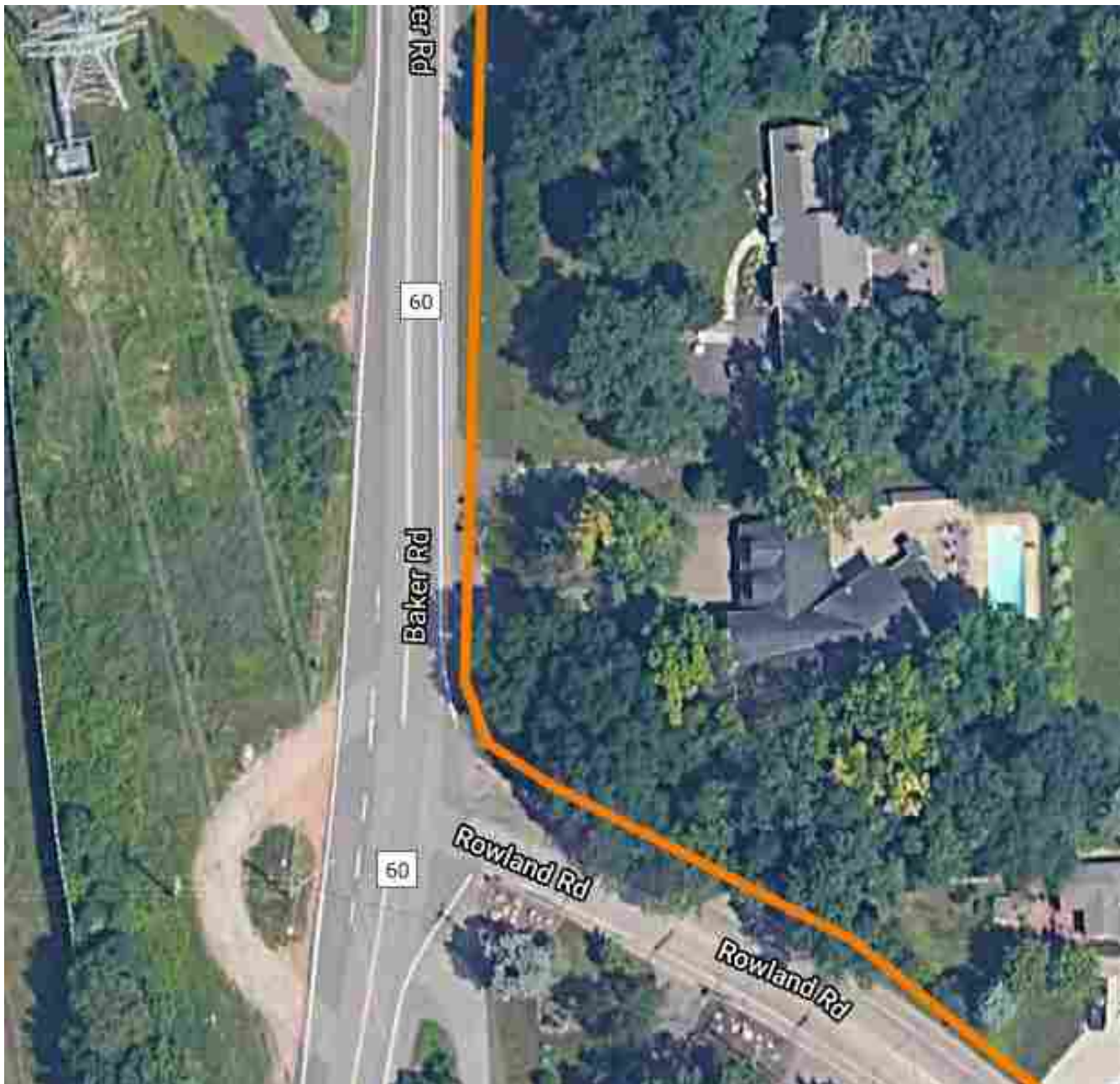
Figure 5: Recommended trail alignment (orange line) at the intersection of Baker Rd and Rowland Rd. The proposed trail is recommended to continue to the east along the north side of Rowland Rd.
