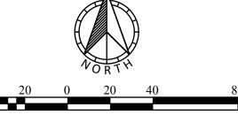
The basis for the bearing system is the north line of Section 08, Township 117, Range 22, and is assumed to bear North 89 degrees 16 minutes 56 seconds East. (See Sheet 2 of 2 Sheets)
