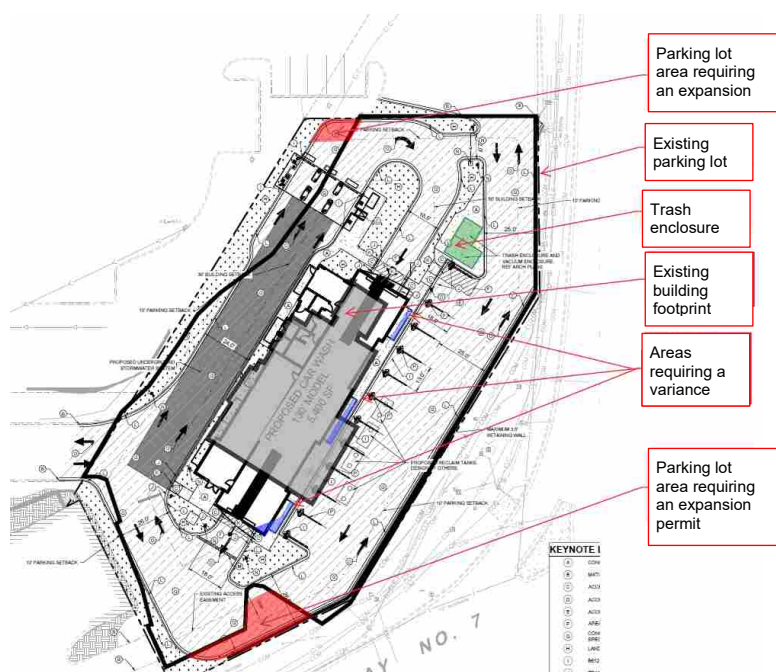
Figure 5: Existing and proposed site improvements
